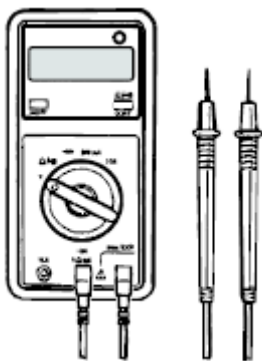
Fig. 3: Identifying Commercially Available Digital Multimeter Courtesy of PORSCHE OF NORTH AMERICA, INC.
