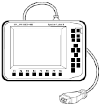
Fig. 2: Identifying 9588 Porsche System Tester II Courtesy of PORSCHE OF NORTH AMERICA, INC.
