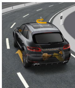
PTV Plus (Porsche Torque Vectoring Plus)
